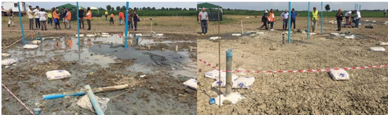
Figure 7.9: Comparison of observable liquefaction effects in the NP (left) after blast 1, and the IP (right) after blast 2 ( http://www.releo.it/blast-test-impact-pier.php ).
